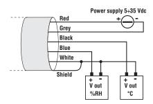
The instrument is equipped with a 7 wire + shield cable.
