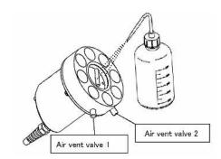
Clean the inside of the measuring cell using pure water. Air vent valve 1 and Air vent valve 2 should be closed.
