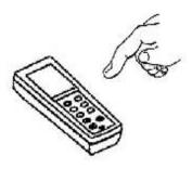
Connect the meter part to the measuring cell. Press the **POWER** key to turn the meter on and press the **MODE** key to get  $\mu$ S/cm units.
