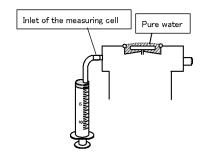
Connect the tube from the syringe to the inlet of the measuring cell and inject the pure water into the measuring cell. Ensure that the measuring cell is inverted to contain the water that has just been injected into it.
