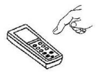
Press the **ZERO** key to perform zero correction. Then press the **MODE** key to get mg/m<sup>2</sup> units.
