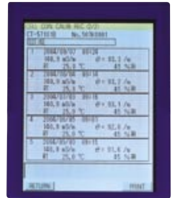
Screen of calibration history of conductivity measurements
