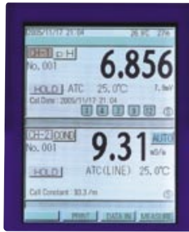
Example of pH / conductivity measurement screen
