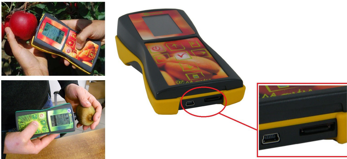
fig.2 – User-friendly case, with tactile keyboard, LCD display to show acquired measures, data storage on a Micro-SD-Card and download on Windows® operating system equipped PC using the proper software and by the rear USB interface.
