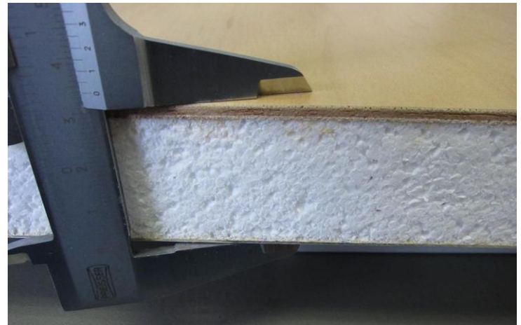
Example sandwich: aluminum - insulation - plywood
