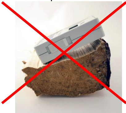
False: wrinkled surface (extreme example!)
