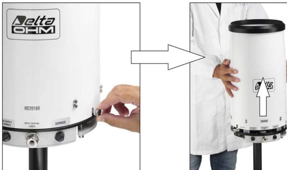
Fig. 9.2: removing the cylindrical cover
