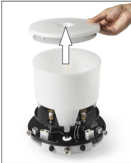
Fig. 9.3: rainfall collecting reservoir
