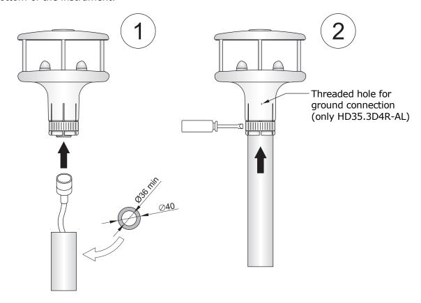
The support mast, having 40 mm maximum outer diameter and 36 mm minimum inner diameter, should be positioned on a stable surface and must be connected to ground.
