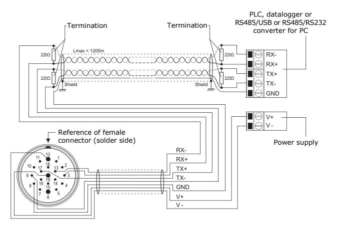
RS422 standard is used for point-to-point connection on long distances. The instrument is connected to a PC/data logger through a shielded cable with two twisted pairs for signals and an additional wire for ground. The extremities of the connections should end with line terminators.
