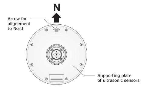
If a magnetic compass is used for alignment, take into account that the geographic North differs from the magnetic North indicated by the compass. The difference, named **magnetic declination**, depends on the area where the instrument was installed (for example, about 15° in North-America and less than 3° in Europe).
