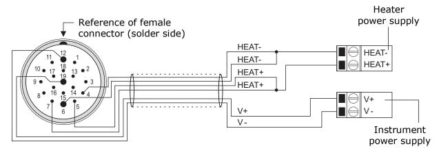
The heat circuit is switched on below  $+4\,^{\circ}\text{C}$ . After switching on, the heating is switched off when the temperature exceeds  $+10\,^{\circ}\text{C}$ .
