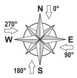
Take into account that the instrument measures the wind direction with respect to the reference arrow on the housing (the instrument is not equipped with a magnetic compass for the automatic compensation of the direction).
