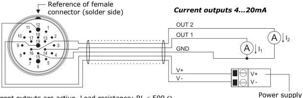
Current outputs are active. Load resistance: RL  $\leq$  500  $\Omega$ .
